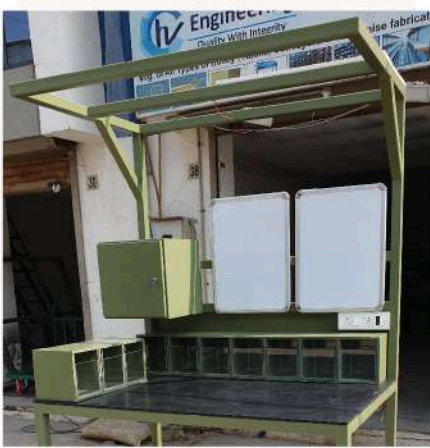
(G-5) ASSEMBLY TABLE FOR VALVE ASSEMBLY
