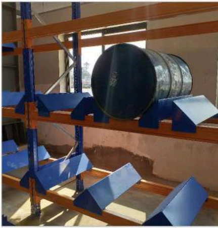
(F-7) DRUM STORAGE RACK
