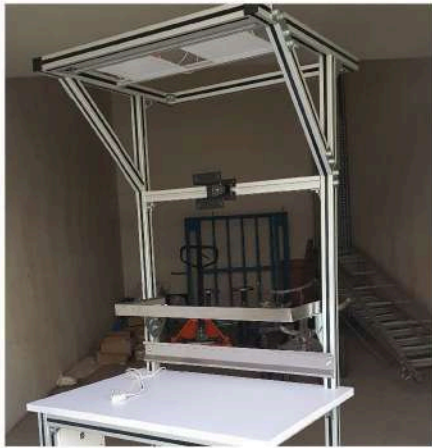
(G-3) ASSEMBLY TABLE FOR ELECTRIC READING METER
